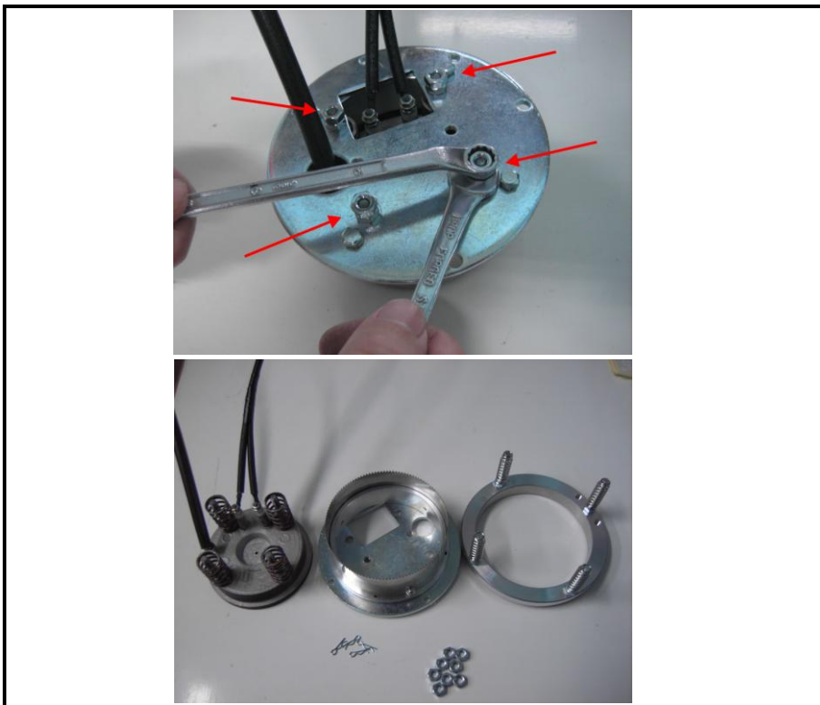
Graph 7-2、3 Using a wrench and box end wrench to separate the knife and heater. Then you can clean the mould and parts.
