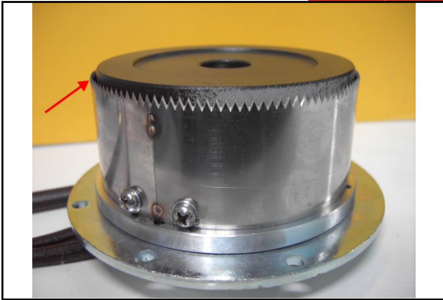
Graph 8-1 After cleaning, heater' s position should be higher than the knife for 1 mm °
