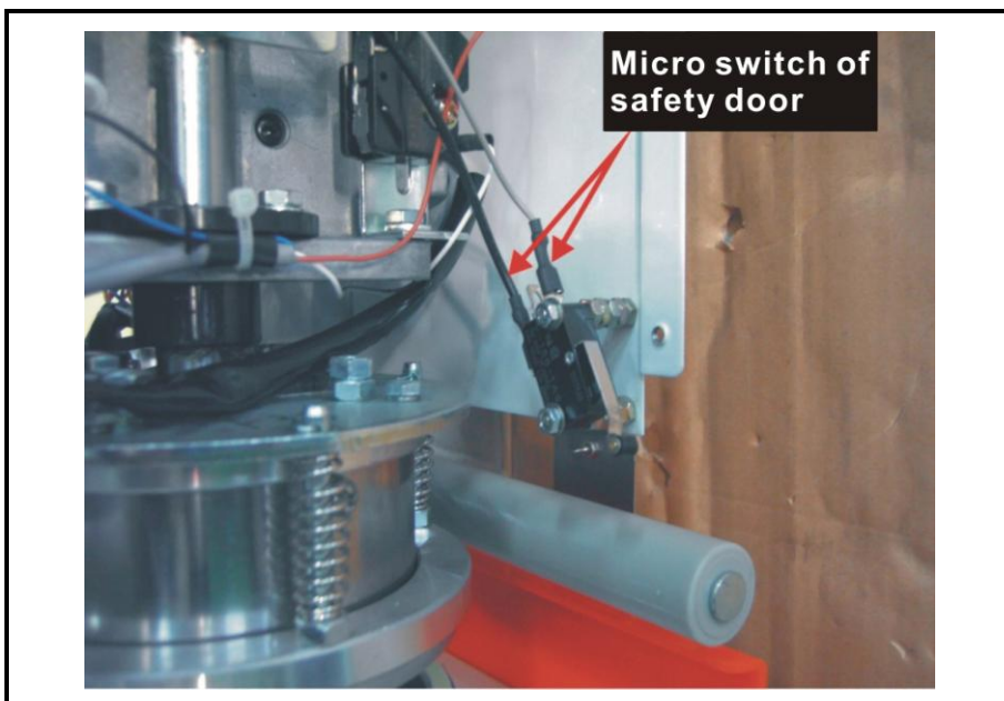
Graph 13-1 For error code E07 : Check if the micro switch is broke.
